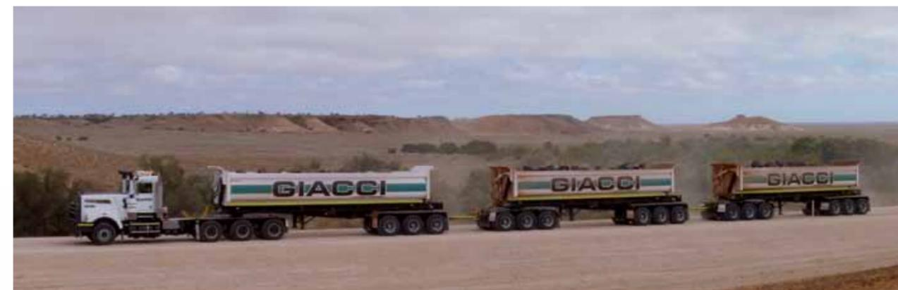
180 tonnes of iron ore rock material. Every combination is pulled by a Kenworth C510 tri-drive prime mover, the largest capacity Kenworth truck available on the market.
